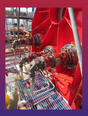
GSM PT UK LTD can supply an "o ffthe shelf" complete winch solution which comprises of a winch drum mounted on a planetary gearbox, with a steel frame/ stand, negative multi-disc brake, hydraulic motor and valve control. All the operator needs to do is fasten the winch down, put the cable on the drum and connect the hydraulics to the power pack.
