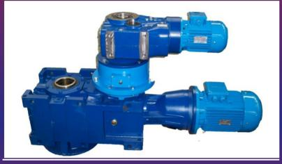
The drive solution shown on the left was specifically designed against the customer's existing circa 1966 obsolete gearbox arrangement. The final output torque is well in excess of 100,000Nm and comprises of 2 separate drives. The central drive is for driving the discharge auger at a speed of 20 rpm. The second drive agitates/mixes the 50T of product at a constant steady rate.
